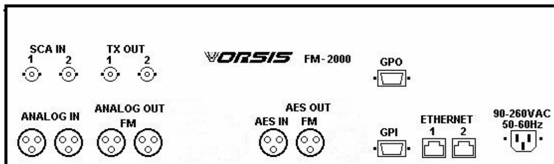
FM-2000 Rear Panel Connections
